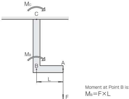
As described above, when the moment is applied to the beam (rod), the moment is the same at any point. Therefore, the moment at Point C is:
