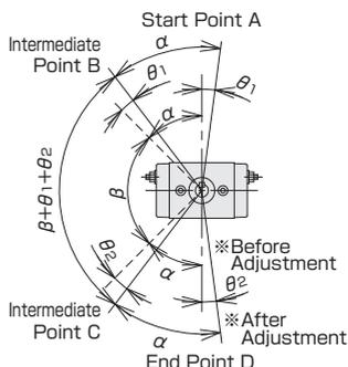
**■ Relationship between Rod Rotation Adjustment Angle and Stopper Bolt A/B Rotation Angle**
